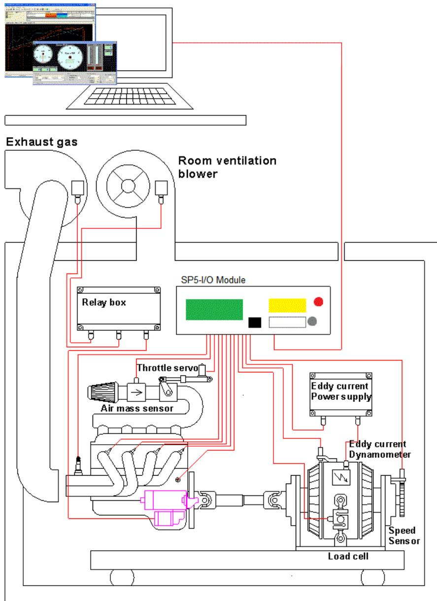
Note: SP5 can be installed close to the dyno / engine to shorten all data and control cables, and then only the serial cable will have to go through the wall to the computer. All control tasks will be performed from the computer, although for safety critical actions (as turning the engine ignition OFF) it is recommended to have an extra switch in series, at the control room.
