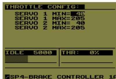
**MIN THROTTLE:** starting position for the servo when THR=0%. In steps of 1/255. You have to ensure the throttle is completely closed at this position (consider engine's idle adjust). In this option both knobs can be used to change the value.
