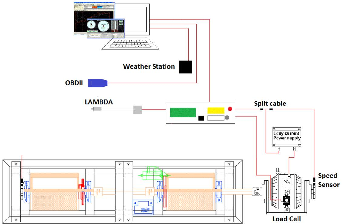
Note: speed sensor can be mounted on rollers or at brake
