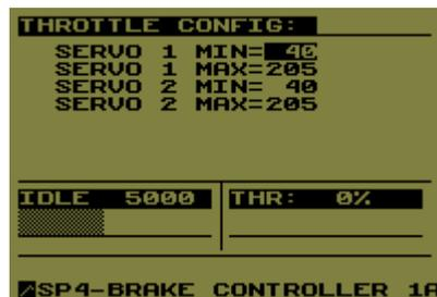
**MIN THROTTLE:** starting position for the servo when THR=0%. In steps of 1/255. You have to ensure the throttle is completely closed at this position (consider engine's idle adjust). In this option the LEFT knob is used to change the value.
