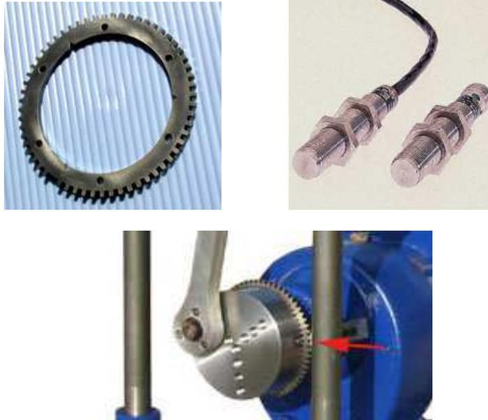
The sensor is thought to be placed horizontally in the machine (3 o'clock = 0 degrees) but if its position is different, it can be configured in the software: "sensor offset". The rotation should be **clockwise**. It can be done by swapping the cables from three-phase motor.
