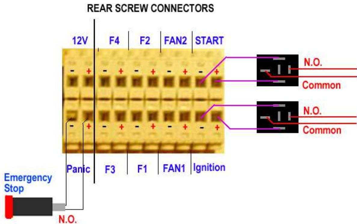
Emergency button is a Normally Open Switch that can be connected to the “panic” terminals. Polarity does not matter. When pressed the SP5 will apply a pre-defined brake torque to the rollers until they are stopped (switch can be released before the rollers are stopped)
