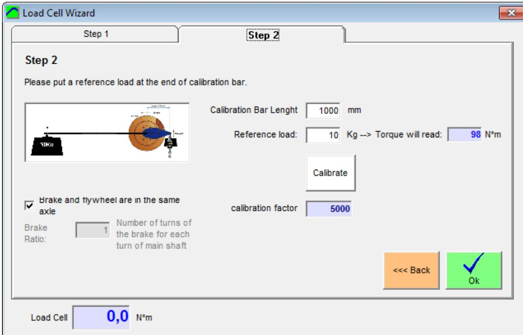
Note: if no calibration arm is available, calibration can be performed directly over the cell arm/lever with the following considerations:
