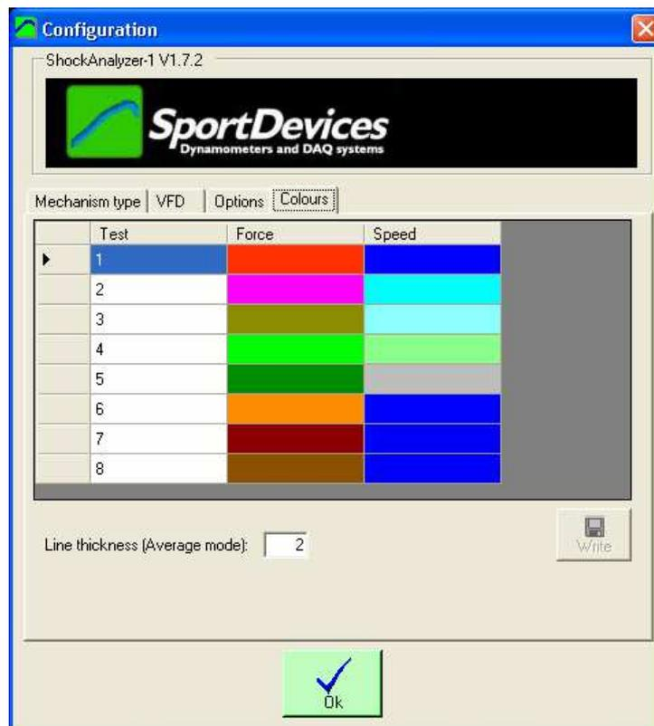
Each channel for each test can have a different colour. The user can edit them on this window. After editing, the **write button** has to be pressed to save the changes.
