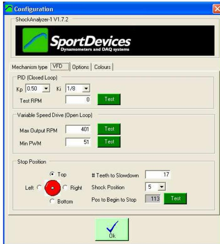
This window is used to configure the VFD (Variable Frequency Drive) output which powers the 3-phase motor.
