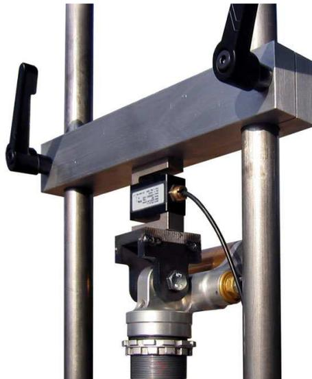
When adjusting the upper bar, the user must ensure that the shock absorber can move along all its displacement and it doesn't reach its boundaries because in such case, the force applied to load cell will be very high and it could be damaged.
