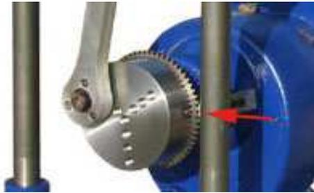
The sensor is thought to be placed horizontally in the machine (0 degrees) but if its position is different, it can be configured in the software: "sensor offset". The rotation should be **clockwise**. You can get it by swapping the cables from three-phase motor.
